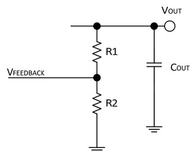
For LDO1, A resistor from the output node to the feedback pin sets the output voltage.
